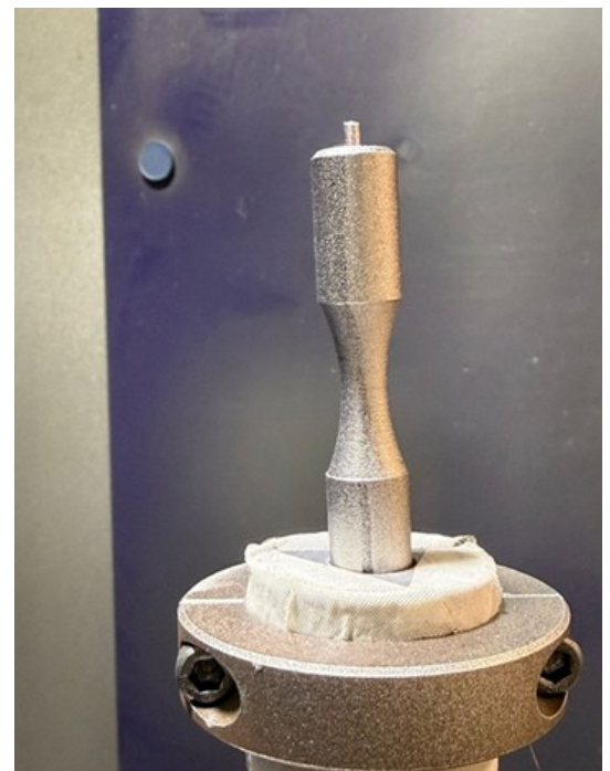
Figure 2. Peened dogbone specimen for fatigue testing.
